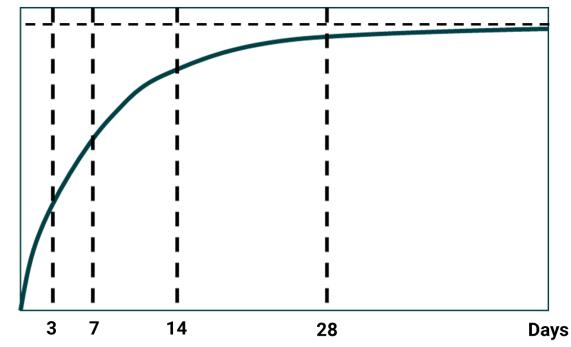
The rate of strength development must be taken into consideration when planning the tests
